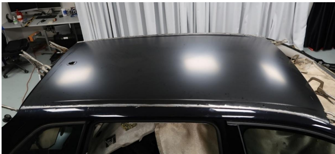
Roof Post Laser Welding
